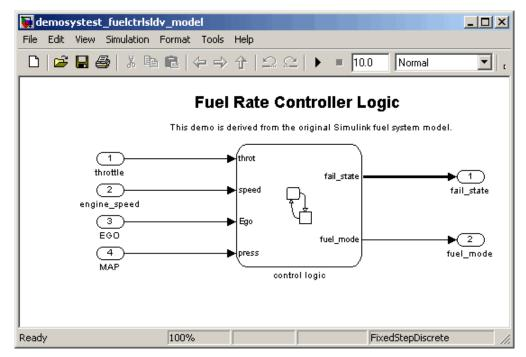
12 In this case, you want to map signals you created in the Test Case Editor to these four Inports in your model. Use the **Override Inport Block Signals with SystemTest Data** section of the Simulink element.
