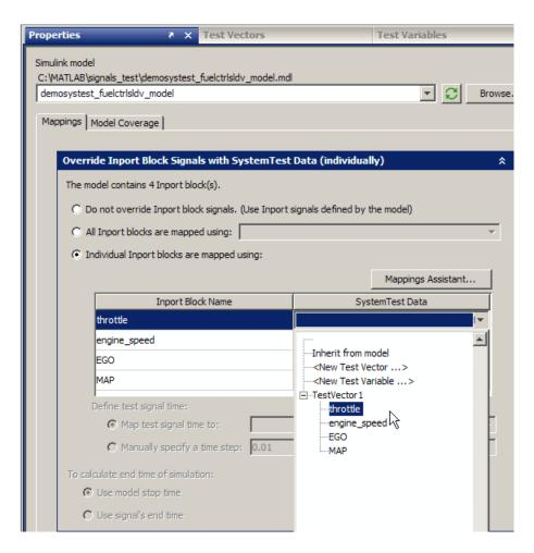
You could also use the Mappings Assistant (click the **Mappings Assistant** button to open it) and select them all at once by selecting the Test Case Data test vector in the **A test case data test vector's signals** override option, as shown next.
