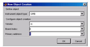
**9** Click **OK** to return to the Edit: Instrument1 dialog box, where the instrument object is now filled in and selected for this resource (GPIBO-5).
